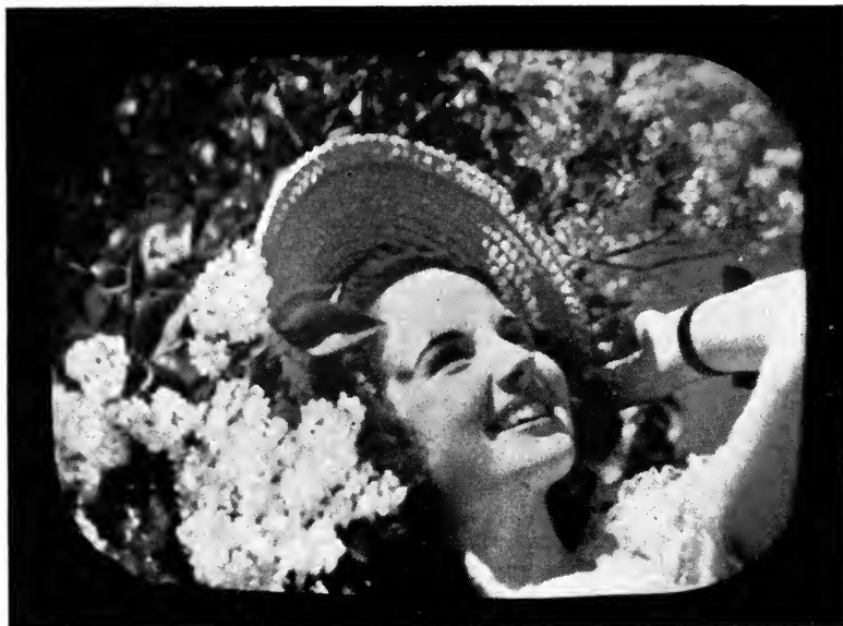
Fig. 8. Picture transmitted with system flat to 10 mc, uncrispended.
